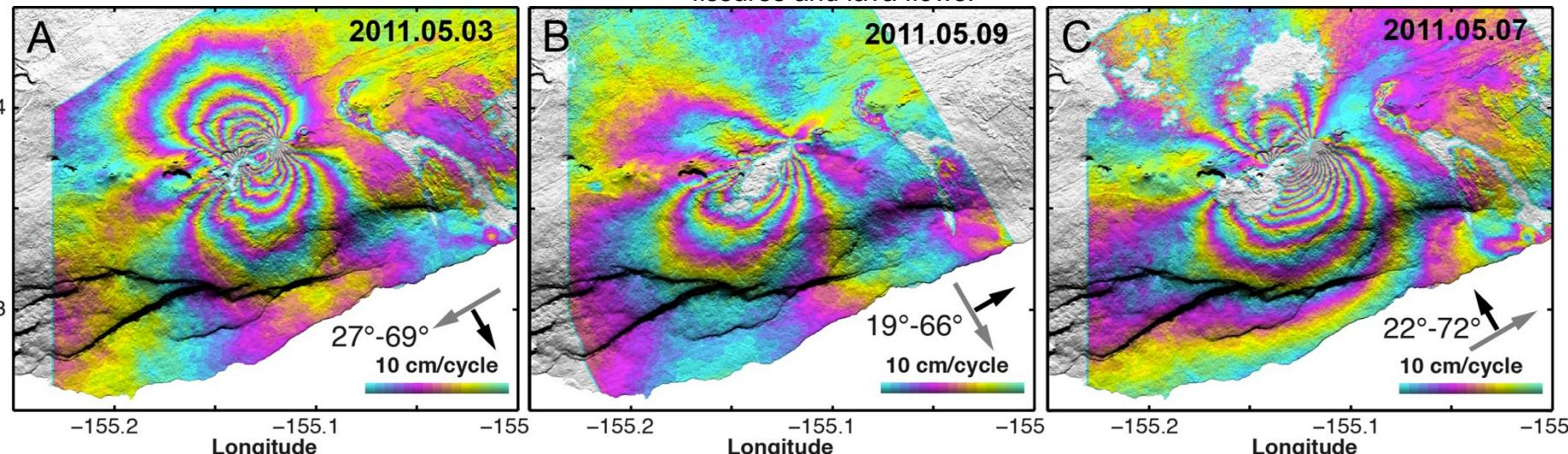
Figure 2. UAVSAR interferograms for the dashed box area in Fig. 1B. Each interferogram is from a different viewing directions as indicated by the aircraft heading (gray) and look direction (black) arrows and their near to far range ground incidence angles.
