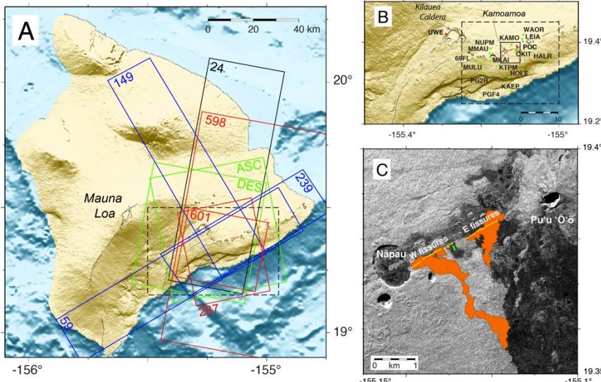
UAVSAR plus satellite InSAR and GPS data were used to constrain the detailed dike opening models and dike volume history shown in the next slide.
