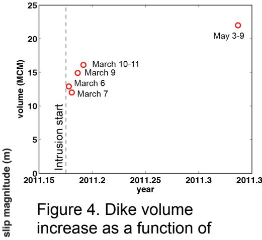
Figure 4. Dike volume increase as a function of time for the dates with InSAR data and models. Following the end of the eruption (March 9) there was continued dike volume increase as shown by the March 10-11 model and the UAVSAR constrained May models.
