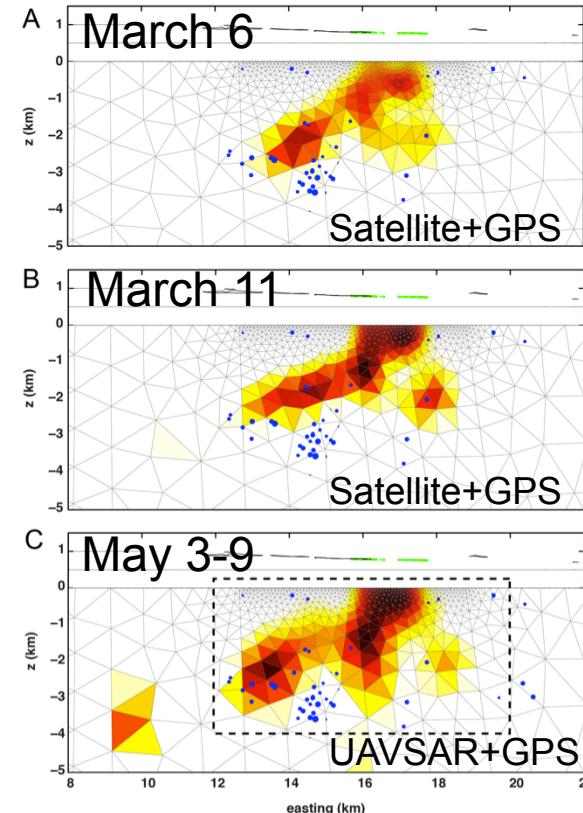
Figure 3. InSAR + GPS constrained model side views of dike opening for three dates: March 6, within 24 hours of the eruption start (ALOS); March 11, after the end of the eruption (ALOS, CSK, TSX); and early May (UAVSAR). The models show growth in amount of opening and area and suggest the dike was fed from its deeper limb plunging to the left and a shallower limb to the right.
