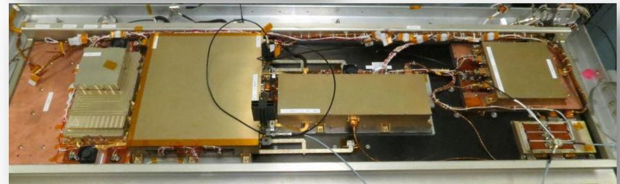
**Ka-band high power amplifier and RF electronics are mounted to the backside of the antenna baseplate**
