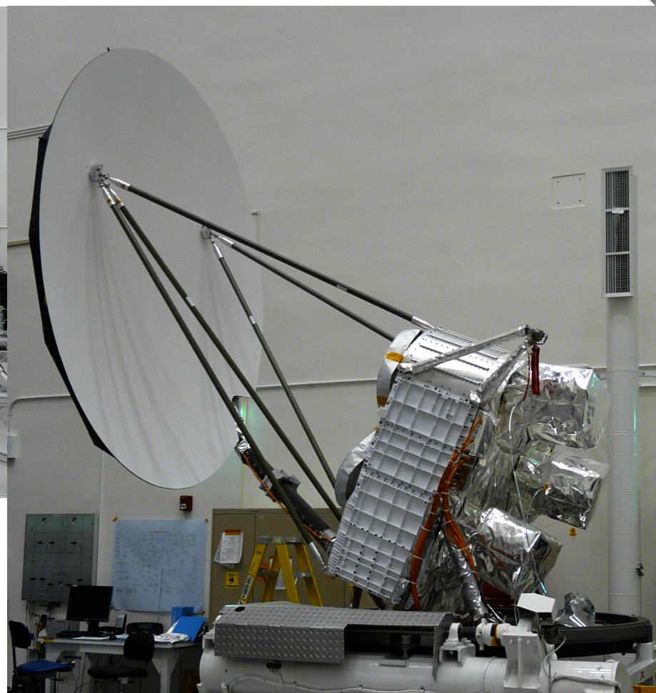
Aquarius instrument in deployed state at JPL. Fiber glass support struts hold the reflector when deployed in gravity environment.
