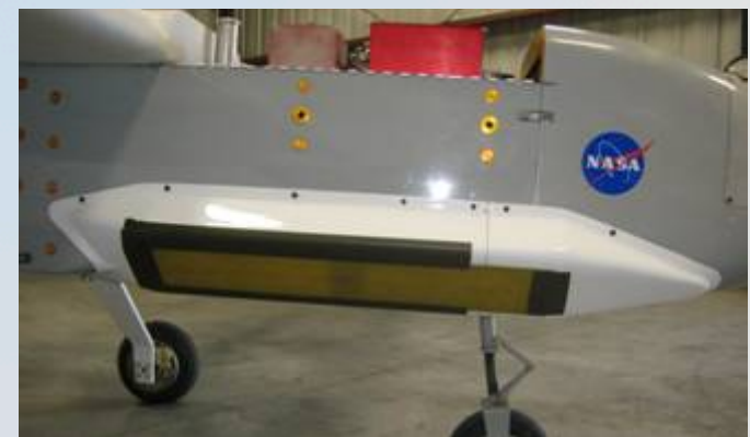
The MicroASAR antennas mounted on the side of the SIERRA
