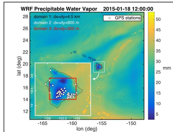
**Figure 2.** WRF model output for January 18, 2015 12 UTC showing the simulated precipitable water vapor (PW) and the 3-domains configuration with their respective horizontal resolutions. The white dots on the Big Island of Hawaii correspond to the locations of the GPS stations used in the custom analysis for the 300 m resolution domain (domain 3).
