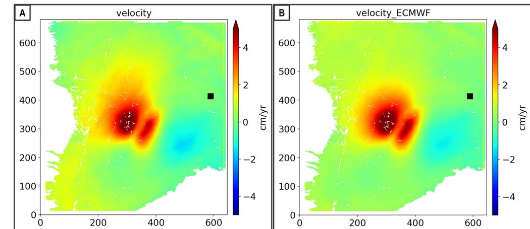
**Figure 4.** Preliminary result of a "velocity map" of the Mauna Loa inflation using InSAR data for 2015-2016 corrected with our custom analysis (A), compared with the default atmospheric correction using ECMWF ERA-Interim (B). Our corrected velocity field shows subtle differences that we are in the process of evaluating and validating.
