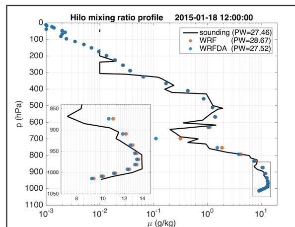
**Figure 3.** Water vapor mass mixing ratio profile at Hilo (Big Island). The black line is the radiosonde data, the red dots are the output from the WRF model and the blue dots from WRFDA (data assimilation). The inclusion of the GPS ZND data and the observations from the MADIS archive brings the total PW of WRFDA closer to the observed value.
