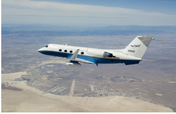
Fig. 2. Modified NASA Gulfstream III in early flight tests with the UAVSAR pod attached to the underside of the aircraft. Photo courtesy of NASA Dryden Flight Research Center.
