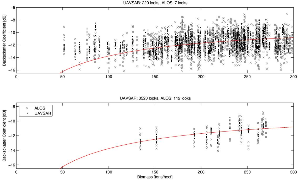
**Fig. 3.** Variation in ALOS and UAVSAR cross-pol backscatter for several datatakes. The ALOS data (FBD, HV), spans a period of over two years (2006 to 2008) with datatakes between July and October, whereas the UAVSAR data spans a period of eight days in August of 2009.
