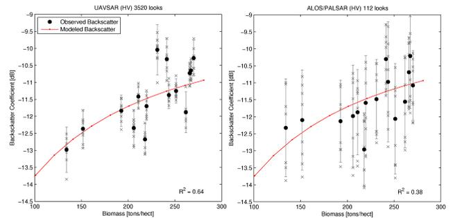
**Fig. 4.** ALOS/PALSAR and UAVSAR cross-pol (HV) backscatter modeled as functions of hectare level biomass estimates. The model and UAVSAR data with 3520 looks are in relatively good agreement with an  $R^2$  value of 0.64.
